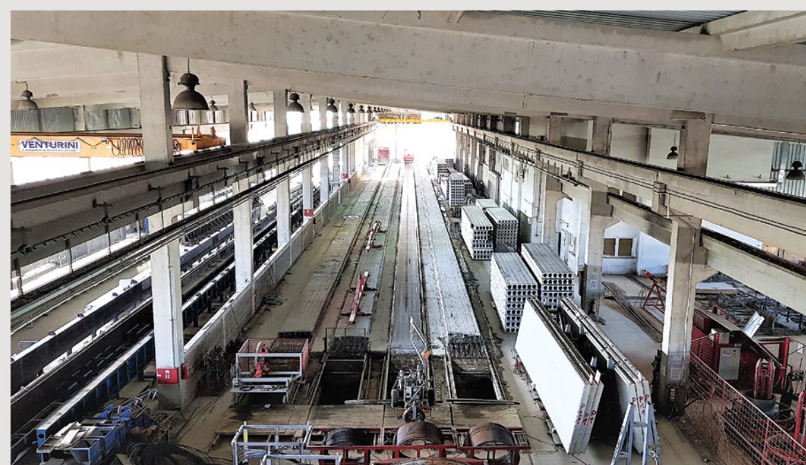
Slika 2. - Pogon za livenje šupljih ploča - Niš / Image 2. - Section for casting hollow plates - Niš
